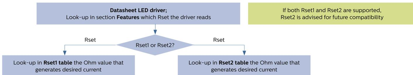
Note on E-series: in electronics, international standard IEC 60063 defines preferred number series for amongst others resistors. It subdivides the interval between subsequent values from 1 to 10 into 6, 12, 24, 48, 96 etc. steps. These subdivisions ensure that when some arbitrary value is replaced with the nearest preferred number, the maximum relative error will be on the order of 20%, 10%, 5%, 1% etc.
