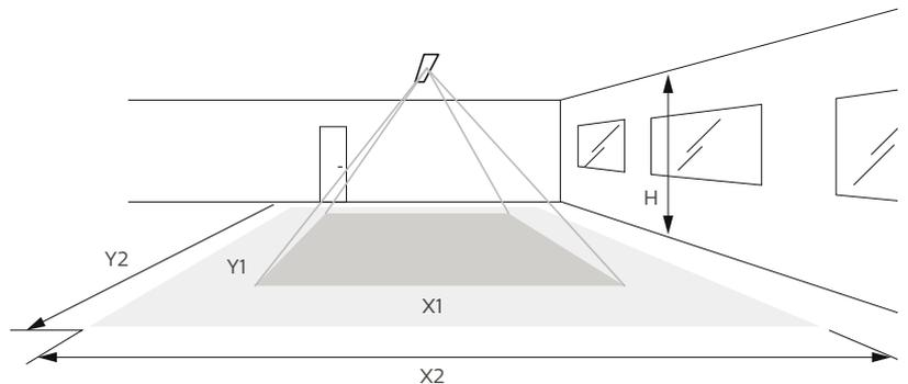
Note: Longer dimension of detection area (Y1, Y2) is parallel to longer dimension of EasyAir SNS200.
