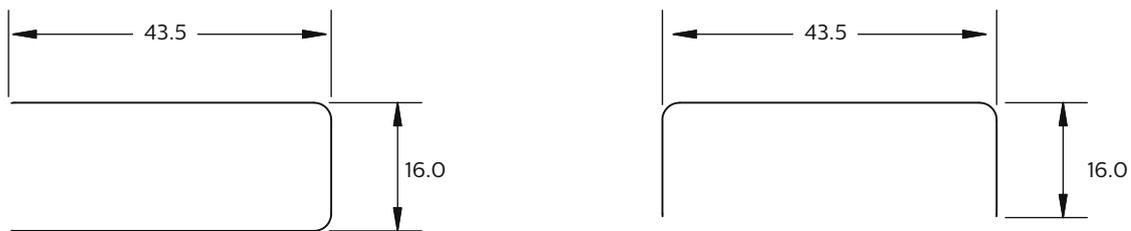
Mounting in cut-out in sheet metal (thickness 0.7 mm to 1.2 mm), tolerance +/-0.2 mm
