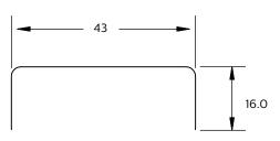
Mounting in cut-out in sheet matal (thickness 0.7 mm to 1.2 mm), tolerance +/-0.2 mm
